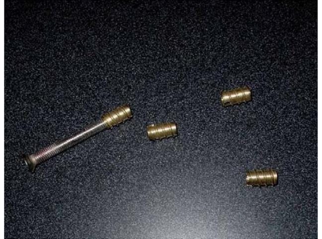
After the launcher is installed on the boat, you will install these brass inserts for the jib blocks. The holes should be drilled oversize ( $3/8$ " for  $1/4$ " OD inserts) and the inserts bedded completely in epoxy. Drill the depth until you feel your bit hit the bottom skin of the launcher. Do not install these block until you have the spinnaker sock ready to install.
