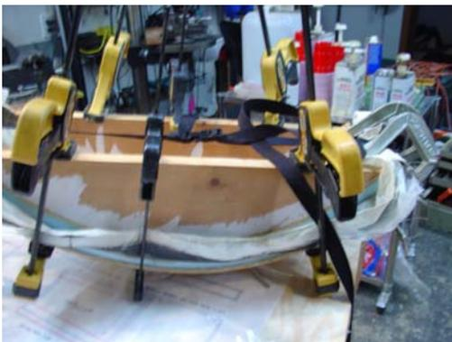
The overhanging lip on the form will eliminate the need for the big clamps shown above, Your clamps will only need a 2 ½ maximum jaw. (sorry for the poor picture)
