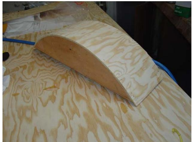
Cut two pieces of  $\frac{1}{4}$  plywood 10" wide and 30" long across the grain of the plywood as shown. Staple or nail one piece of plywood on the forms allowing it to hand over each form 1" (not as shown—but better)
