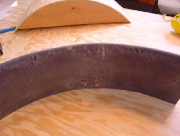
When the part has cured, remove it from the form and remove the peel ply. Sand and fill any imperfections, cover the filler with peel ply and leave it until you bond it to the boat. When you finish your deck you can finish the launcher throat at the same time
